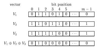
Figure 4: Sample Bit-Vectors for t = 2, p = 1
